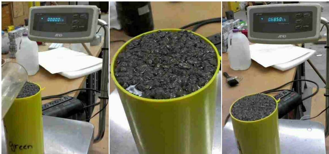
Figure 3.8. Images of porosity testing process
