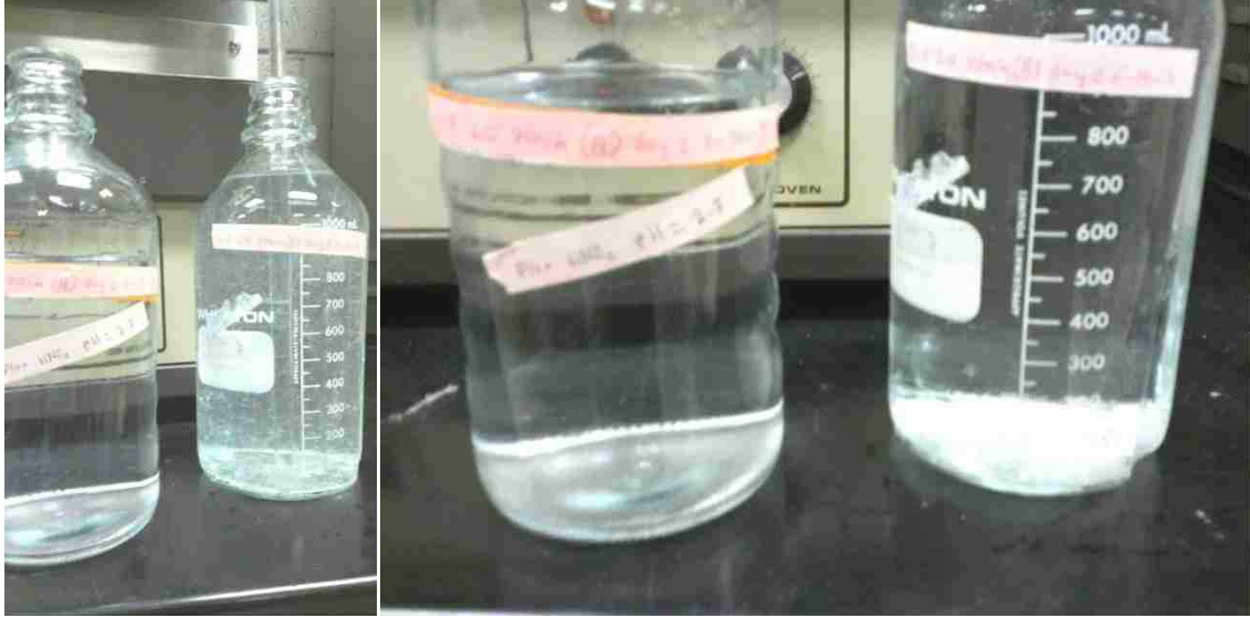
Figure 4.2. Plain A Day 2 samples: acidified (bottles on left of pictures), non-acidified (bottles on right). Picture on left shows samples after stirring, picture on right shows samples without stirring.
