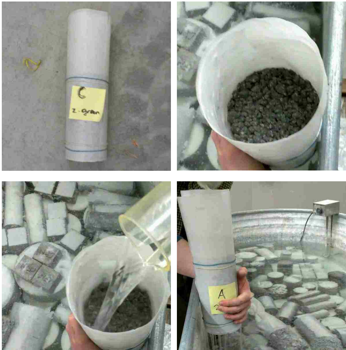
Figure 3.9. Various stages of the permeability testing process
