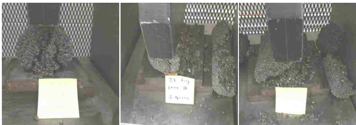
Figure 3.15. Select tensile test failures for (from left to right) plain, 5% and 10% PC
