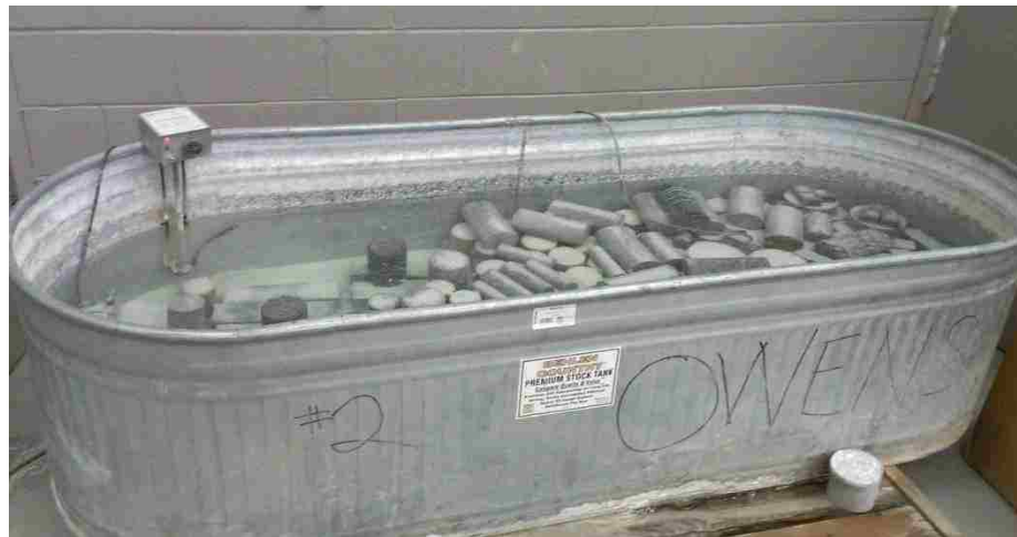
Figure 3.4. Concrete curing tank
